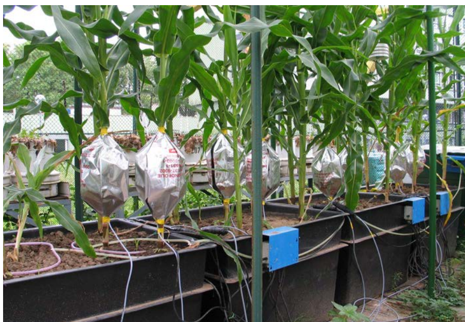
Figure 1: Sap flow measurements of maize by EMS 62 sensors
